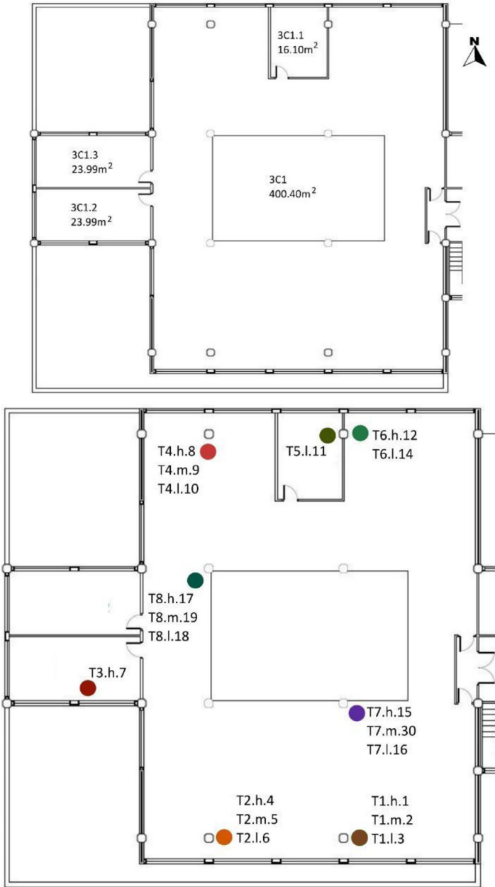
Fig. 11. OT4 sensor layout, located in F3. Based on A2PBEER project's architecture plans [2].
