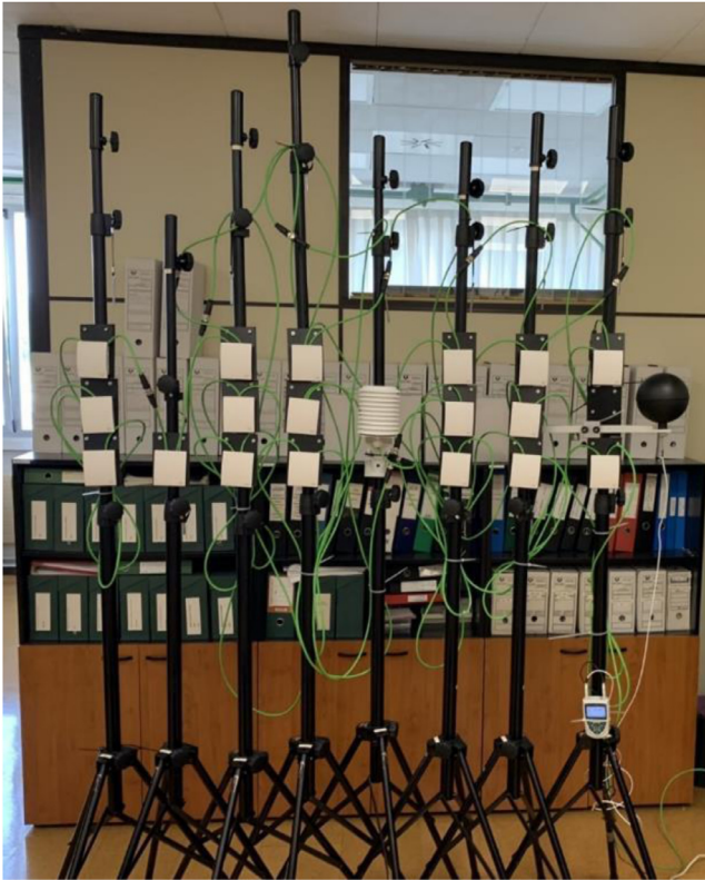
Fig. 7. Interior 3D MMS tripods and sensors all together during the TT test.
