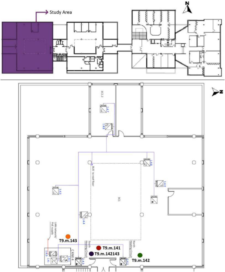
Fig. 5. F3 of the UPV/EHU admin building in Leioa, including the position of the three selected measurement points of the existing BAS referred to in Table 3. Note that T9.m.142/143 is the signal created by adding the measurements T9.m.142 and T9.m.143. Based on A2PBEEER project's architecture plans [2].
