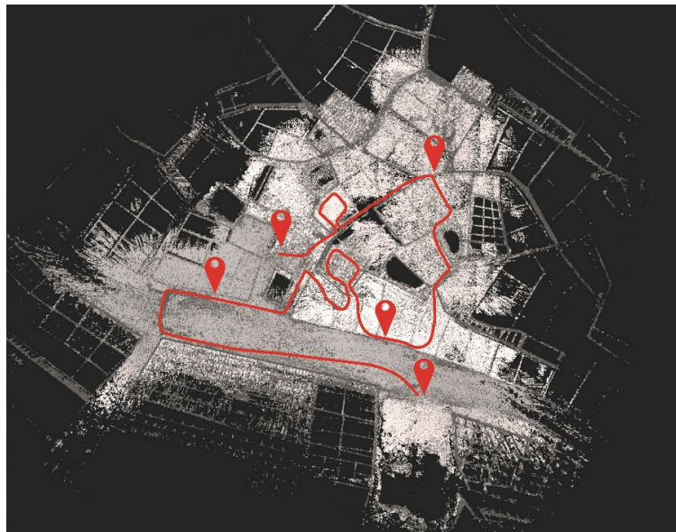
Figure 4. Scan path, real-time point cloud, and detail photo position (Source: Authors).
