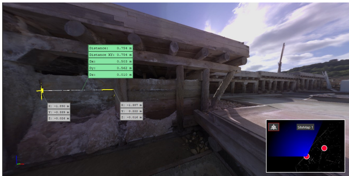
Figure 15. 360° panoramic view of the exterior of the salt pans, with the option of obtaining coordinates and distances, in JetStream Viewer (Source: Authors).
