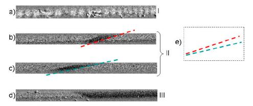
**Figure 5.** Images of different domain structures obtained in the presence of stress observed for different amplitude of torsion  $\tau$ : (a)  $0 \pi \text{radm}^{-1}$ , (b)  $20 \pi \text{radm}^{-1}$ , (c)  $30 \pi \text{radm}^{-1}$ , (d)  $40 \pi \text{radm}^{-1}$ ; (e) schematically images of spiral structures. Reprinted with permission from [17].
