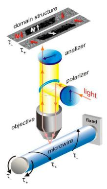
**Figure 1.** Schematic picture of MOKE geometry and application of torsion stress t<sub>+</sub> and t<sub>-</sub>. Reprinted with permission from [36].
