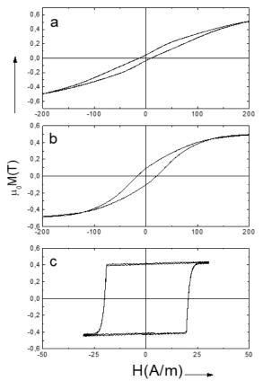
**Figure 13.** Hysteresis loops the microwire N<sup> $ext{e}$ 6. (a) x = 0.08, (b) x = 0.09, (c) x = 0.1. Reprinted with permission from [45].</sup>
