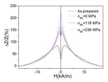
**Figure 9.** Dependencies of GMI ratio on different value of the external tension stress measured at 200 MHz. Reprinted with permission from [5].
