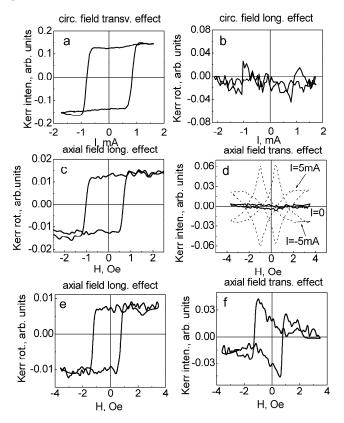
**Figure 14.** Longitudinal and transverse Kerr effect loops of microwire No6 for different Mn content: (**a**,**b**) x = 0.07; (**c**,**d**) x = 0.11; (**e**,**f**) x = 0.09. Reprinted with permission from [37].
