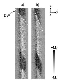
**Figure 3.** MOKE images of surface magnetic domains. Torsion strain  $2\pi radm^{-1}$ . Amplitude of circular magnetic field with amplitude: (**a**) 0, (**b**) 7 A/m. White line shows the inclination of domain walls. Reprinted with permission from [15].
