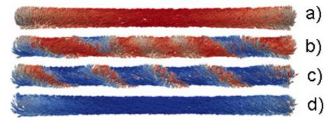
**Figure 15.** Calculated magnetization reversal curve and the images of spiral domains in cylinder with 1 µm diameter and 15 µm length. Images (**a**–**d**) correspond to the points (**a**–**d**) in the hysteresis. Electric current is 1 mA.
