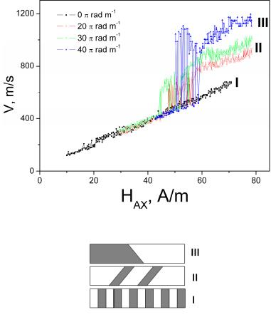
**Figure 4.** Dependencies of velocity of domain wall on axial magnetic field for different values of torsion stress  $\tau$  and schematic images demonstrate three types of domain structure. Reprinted with permission from [17].
