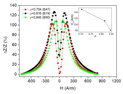
**Figure 11.** Effect of the sample geometry on magnetic field dependence of giant magnetoimpedance effect (GMI) ratio of microwires No4. Reprinted with permission from [19].
