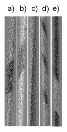
**Figure 2.** MOKE images of surface magnetic domains. Torsion strain: (a)  $-8 \pi \text{ radm}^{-1}$ , (b)  $-2 \pi \text{ radm}^{-1}$ , (c) 0, (d)  $2 \pi \text{ radm}^{-1}$ , (e)  $8\pi \text{ radm}^{-1}$ . Reprinted with permission from [15].
