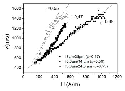
**Figure 10.** Magnetic field dependences of DW velocity for sample No2 microwires with various  $\rho$  ratio. Reprinted with permission from [6].
