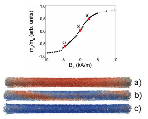
**Figure 16.** Calculated magnetization reversal curve and the images of spiral domains in cylinder with 1  $\mu$ m diameter and 15  $\mu$ m length. Images (**a**–**c**) correspond to the points (**a**–**c**) in the hysteresis. Electric current is 7 mA.
