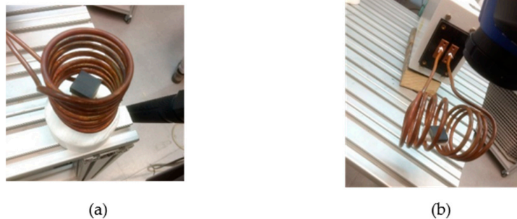
Figure 11. Photographs of the sample inside the coil for different orientations of the Cu slab with respect to the sample surface (painted in black): (a) \varphi < 45^\circ and (b) \varphi > 45^\circ .
