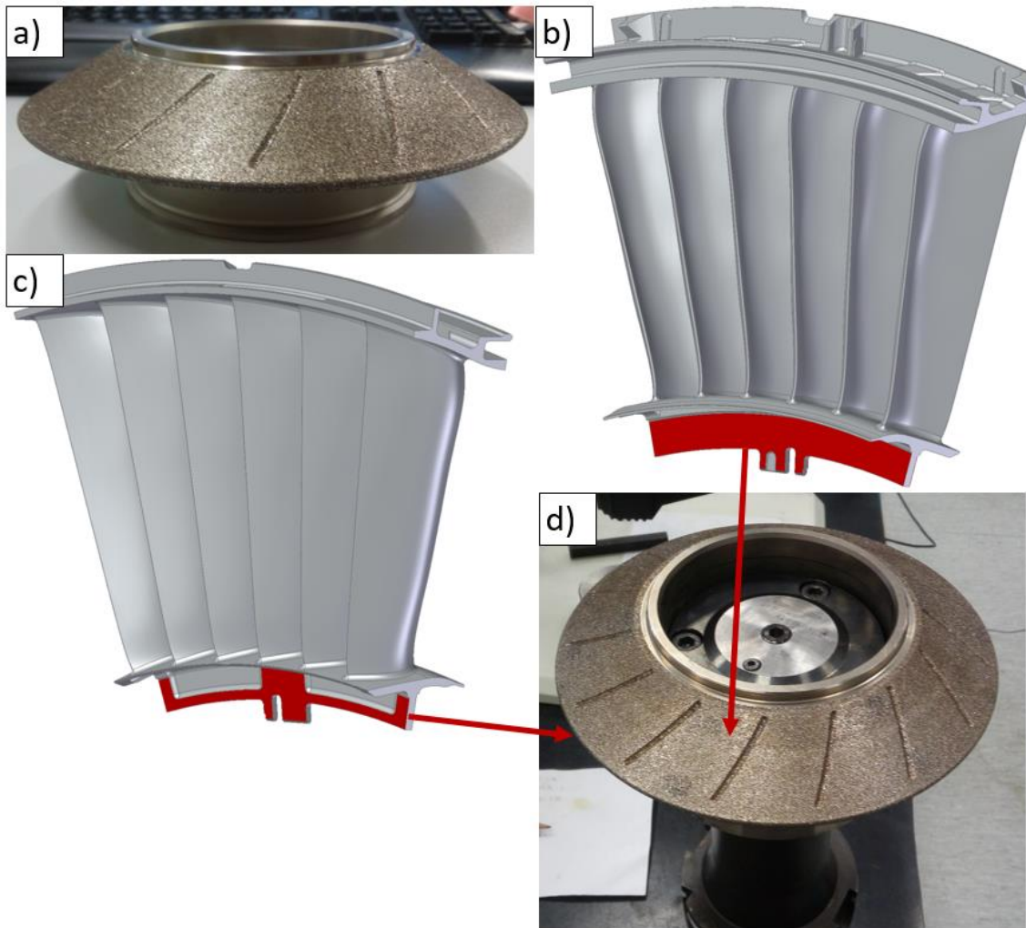
Fig. 63 a) The wheel responsible of grinding the inner rail. b) and c) the two sides of the inner rail marked in red. d) The conical wheel with two differentiated zones as a consequence of the wear.
