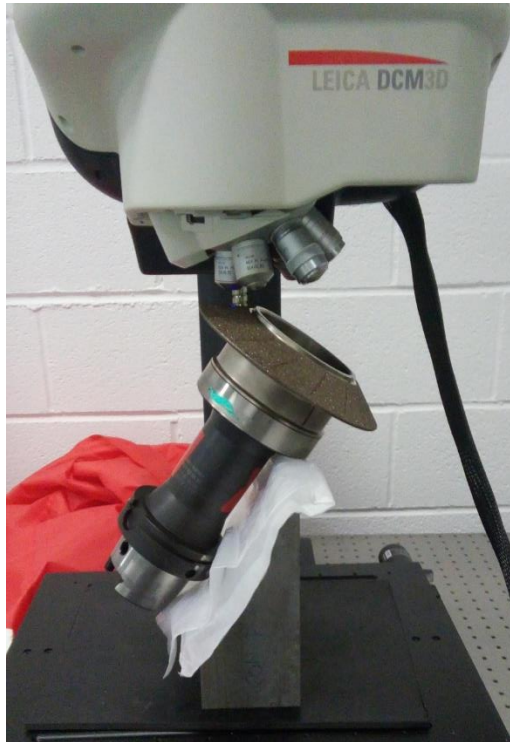
Fig. 64 A conical wheel on the table of the confocal microscope during the digitalization process.
