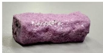
Fig. 102 An alumina pin used for grinding the disk surface.
