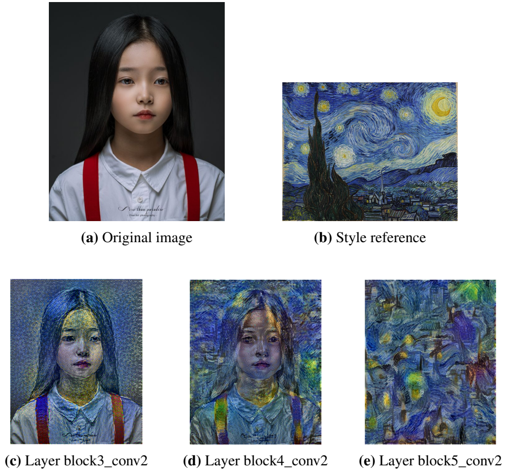
Figure 9.1: Results obtained using different layers to capture the original image’s features after 15 iterations. It can be seen that when using the layer that is nearest to the output layer the original image’s content is completely lost (e). However, using the layer from a block that less deep as block 3, the content of the original picture is more conserved, but the details of the painting are less visible (c). The layer that combines both images in a more balanced way is the second layer of the fourth block, obtaining both the style reference and the base image’s content recognizable (d). The style reference painting is The Starry Night by Vincent van Gogh.
