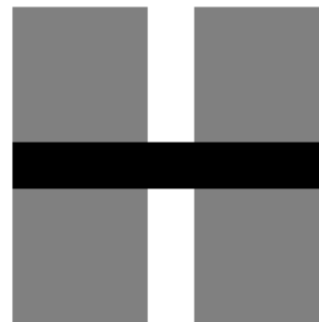
Figure 4.1: 7x7 kernel used for horizontal line detection.
