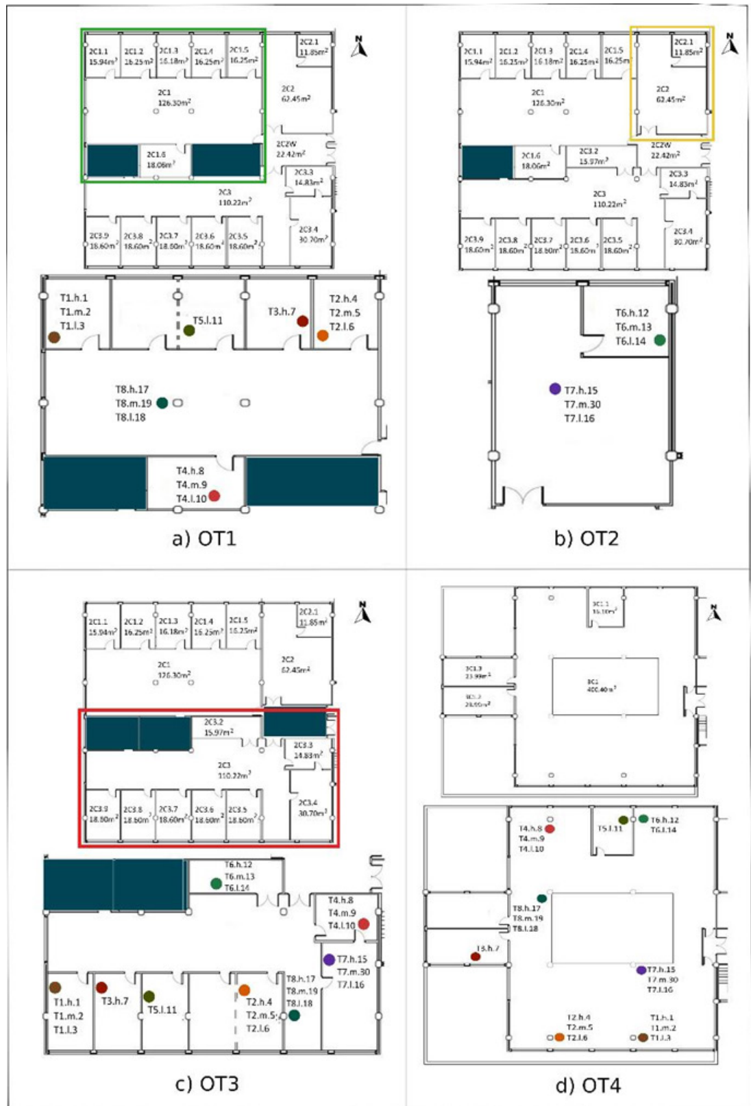
Figure 02. Sensor Layout of Office Typologies (OT) Tests: a) OT1, b) OT2, c) OT3 and d) OT4.
