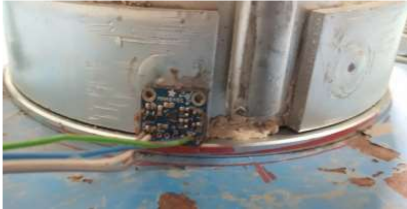
Fig. A1.0.2. Accelerometer sensor positioned on the lower zone of the mould.
