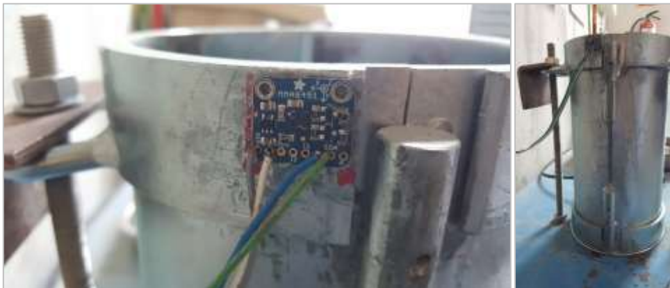
Fig.A1.0.1. Accelerometer sensor position on the upper zone of the mould.
