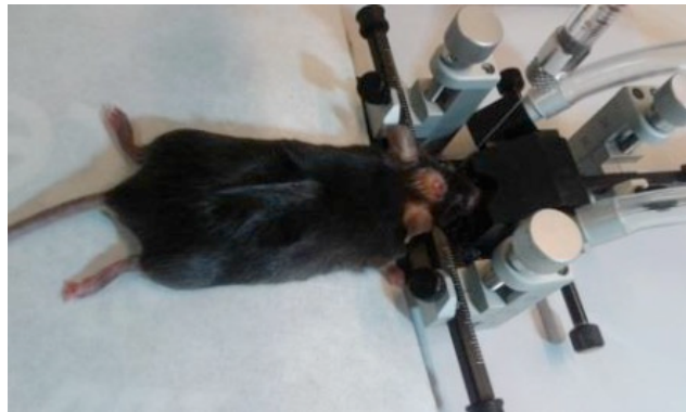
Figure M1. Representative images of stereotaxic instrument (Kopf Instruments) and injection.
