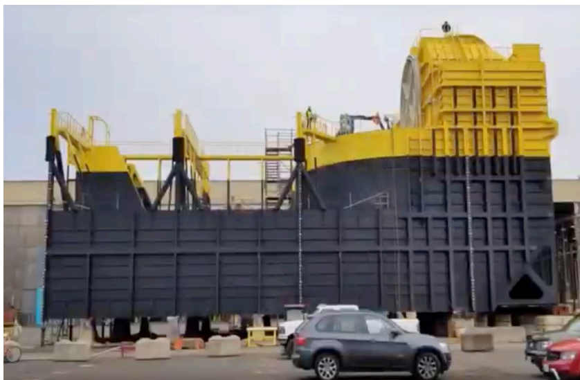
Fig. 2.30: The OE buoy construction in Portland shipyard for installation in Hawaii, photo credit oceanenergy.ie
