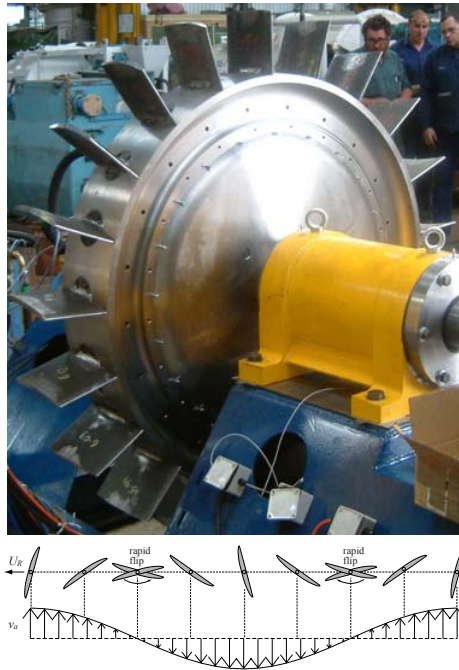
Fig. 2.33: The Dennis-Auld turbine with a schematics of the pitching blades at the top, from [TD03]
