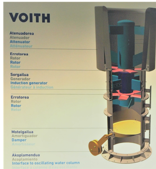
Fig. 2.32: The Wells turbine of Mutriku #3 (photo taken at the power plant)
