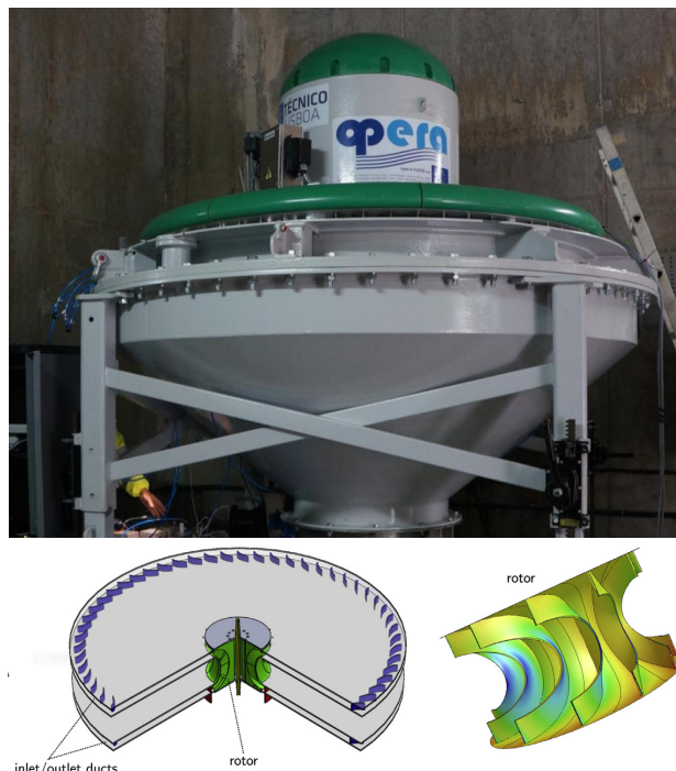
Fig. 2.36: The biradial turbine installed in the Mutriku OWC plant and a schematic of the turbine with guide vanes at the stator outer rim [Hen+16d]
