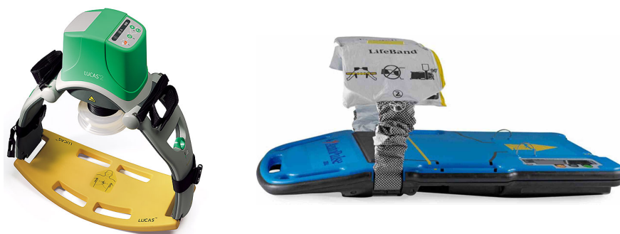
Figure 1.6. The LUCAS-2 and AutoPulse devices. The LUCAS-2 uses a pneumatically driven piston to compress the patient's chest whereas the AutoPulse uses a distributing band placed around the chest to deliver the chest compressions.
