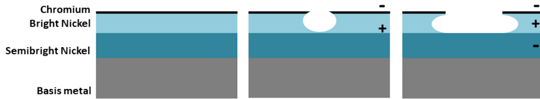
Figure 1.3.- Corrosion mechanism of duplex nickel-chromium coatings.
