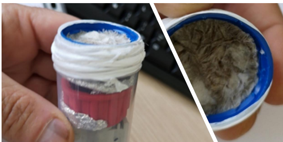
Figure 77 Assembly for permeability tests.
