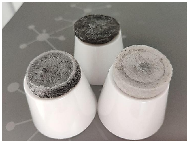
Figure 78 CNC-ALG aerogels loaded with (a) Pd-ZnO (b) Pd-CuO and (c) Ag-CoO metal oxide and metal nanoparticles.
