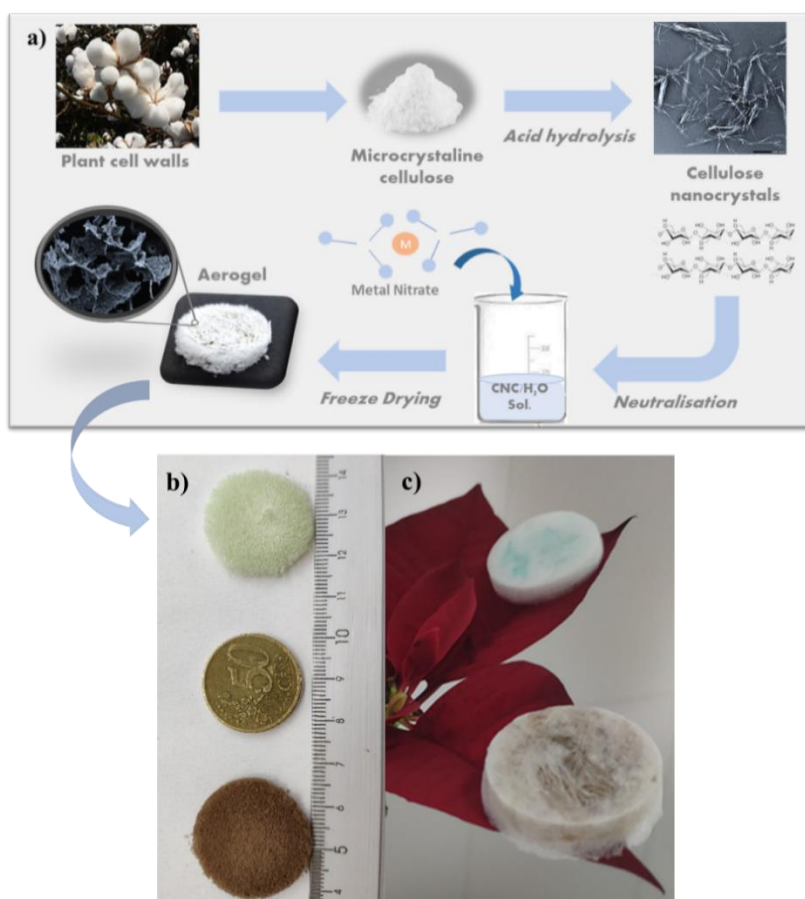
Figure 60 Illustration of the preparation of CNC/MOx hybrid aerogels (a) images of CNC/CuOx, and CNC/PdOx low aerogels (b) and CNC-ALG/CuOx, CNC-ALG/PdOx aerogels (c)
