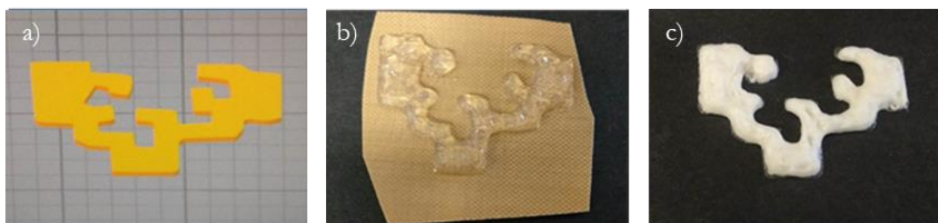
Figure 7.1 Process of preparation of WBPUU0.5 is based shape customized scaffold. From left to the right: a) CAD design, b) printed piece and c) final piece after freeze drying process
