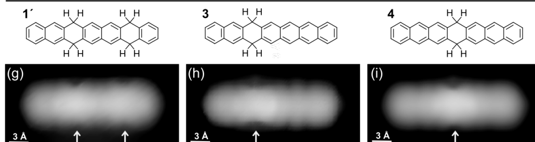
Figure 5.1.3: On-surface synthesis process of heptacene from Br-1, displaying the evolution of the molecule's chemical structure throughout the reaction with two, one, and no hydrogenated non-aromatic rings. The associated high resolution and constant height images revealing the bonding structures ( U = 2 mV, Laplace filtered) are shown in panels (a), (b) and (c), respectively. Panels (d), (e) and (f) display the corresponding constant current STM images ( U = 30-50 mV/ I = 100 pA), while (g), (h) and (i) display the intermediates involving methylene transposition. All images are recorded with CO-functionalized probes.
