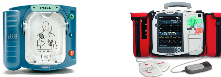
Figure 1.3. Heartstart OnSite HS1 (Philips) AED (left) and Heartstart MRx (Philips) monitor/defibrillator equipped with the defibrillation pads and the CPR aid pad for chest compression feedback (right).
