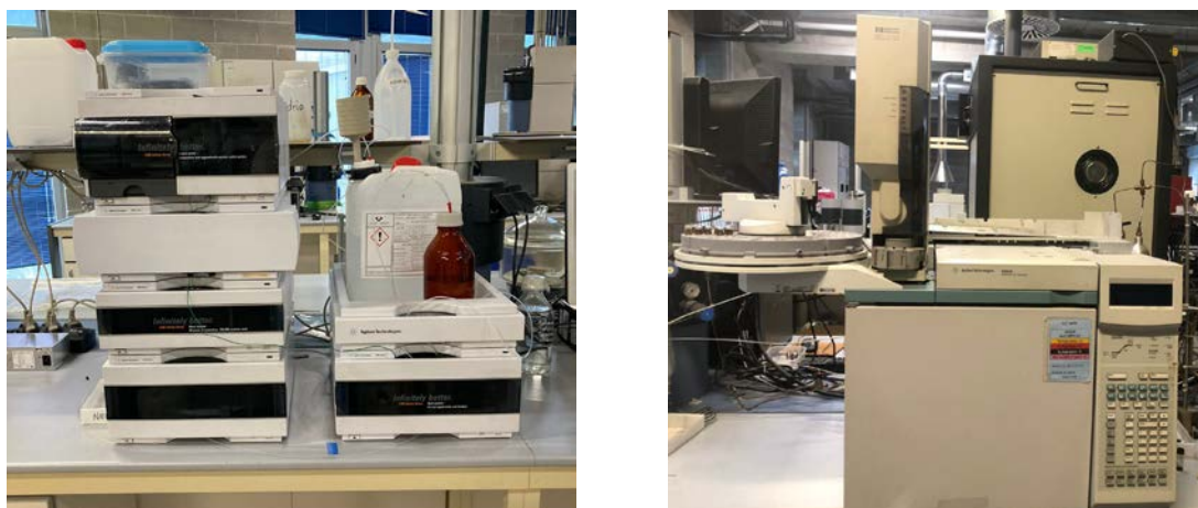
Figure 4.3. Chromatographs employed in the analysis: HPLC (left) and GC-FID (right)
