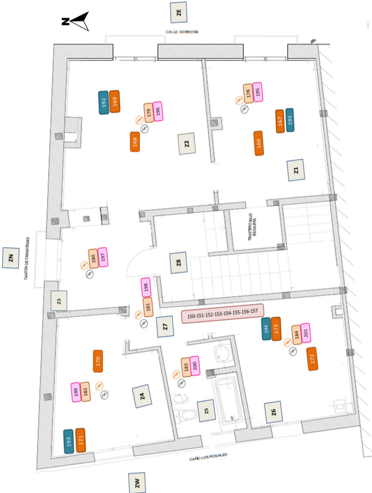
Figure D.6: Sensor Layout of Mobile MCS in F1 for Co-Heating test.
