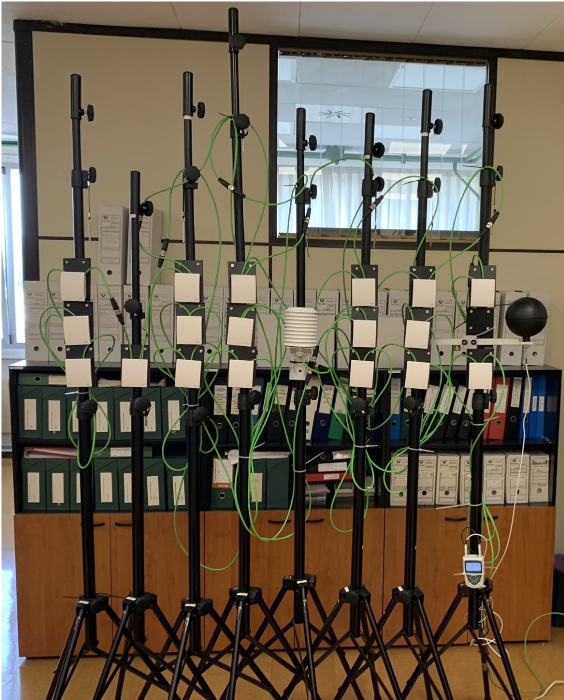
Figure A.5: Interior 3D MMS tripods and sensors all together during the TT test [139].
