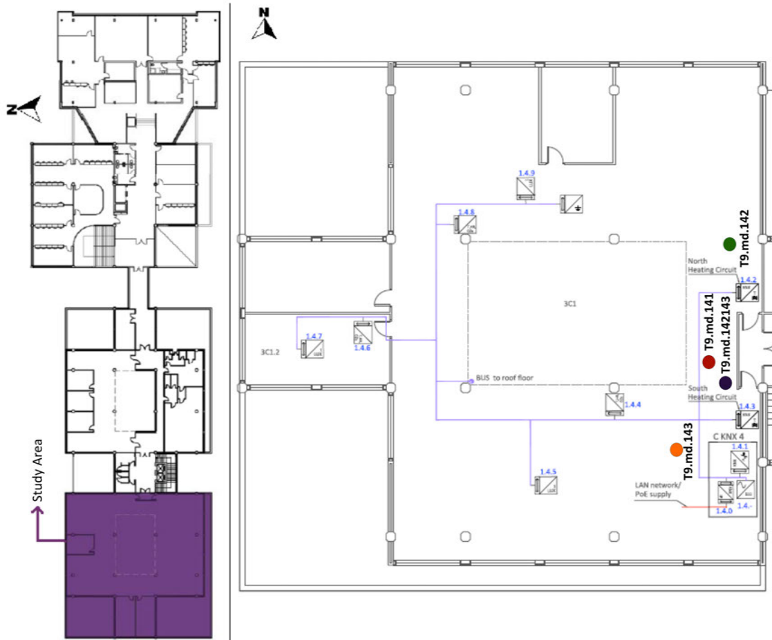
Figure A.4: F3 of the UPV/EHU admin building in Leioa, including the position of the three selected measurement points of the existing BAS referred to in Table A.6. Note that T9.md.142143 is the signal created by adding the measurements T9.md.142 and T9.md.143. Based on A2PBEER project's architecture plans [76].
