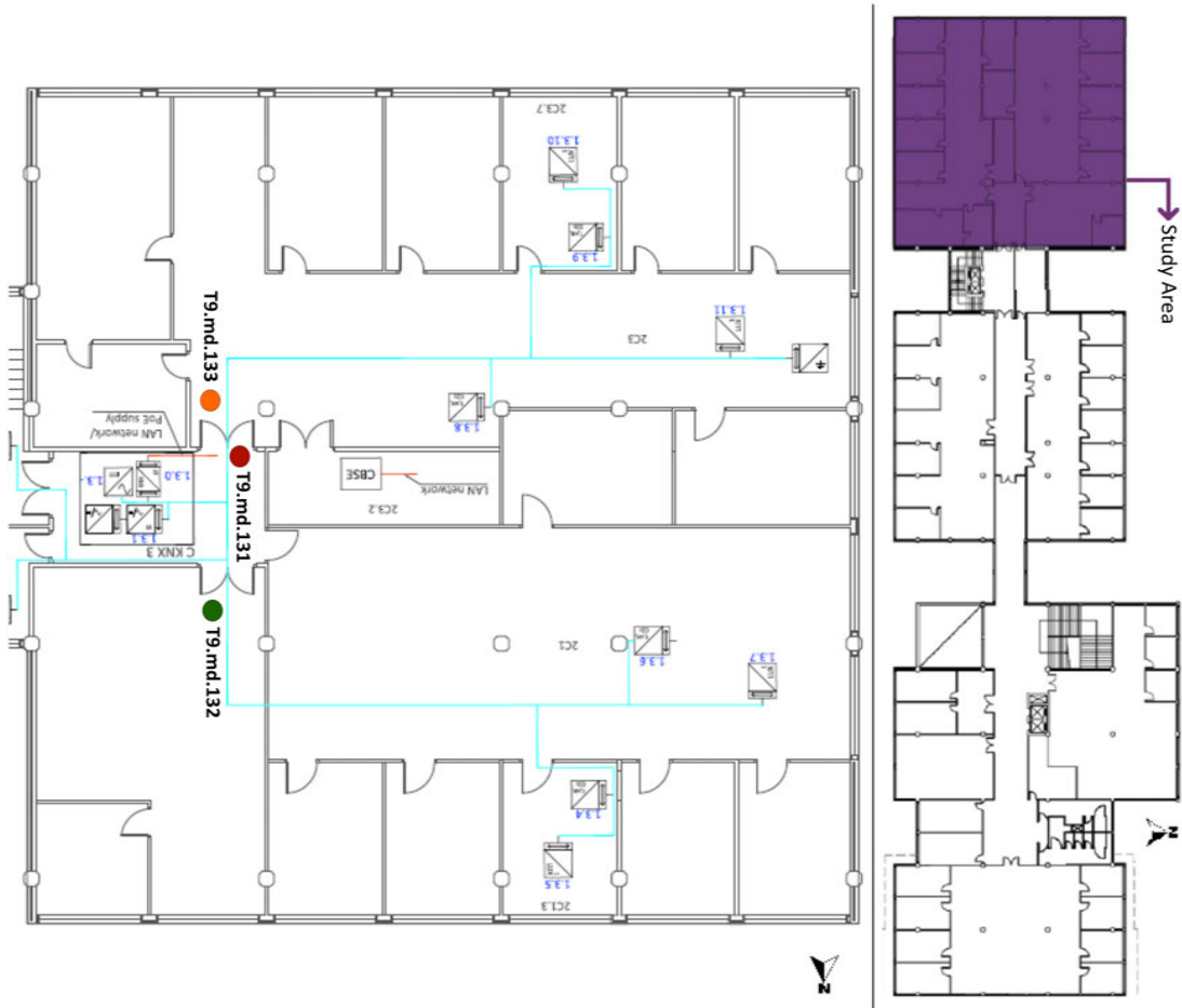
Figure A.3: F2 of the UPV/EHU admin building in Leioa. Includes the position of the three selected measurement points of the existing BAS referred to in Table A.6. Based on A2PBEEER project's architecture plans [76].
