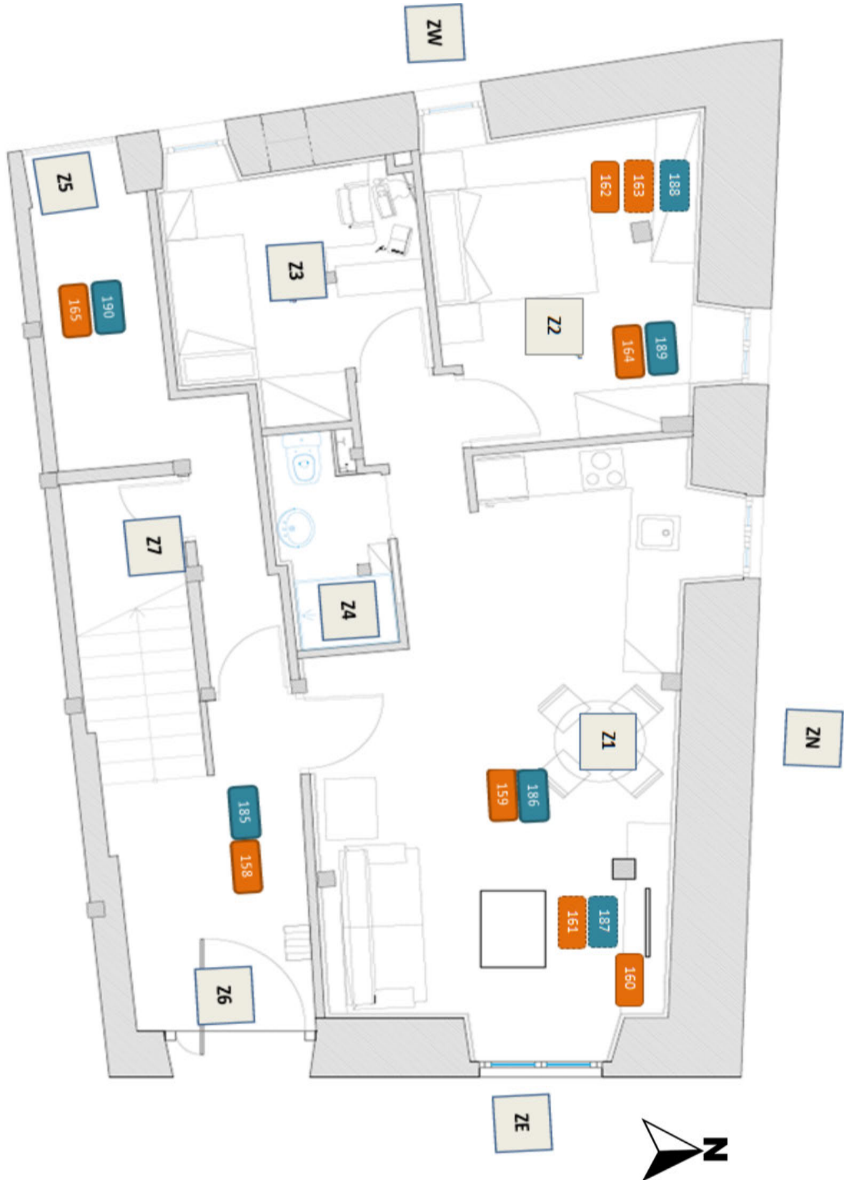
Figure D.5: Sensor Layout of Mobile MCS in F0 for Co-Heating test.
