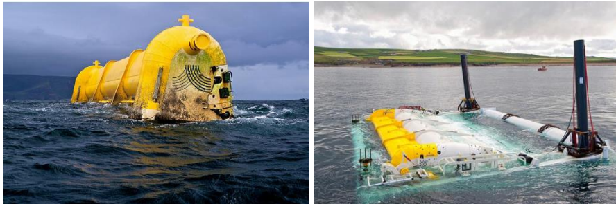
Figure 4 Aquamarine power’s Oyster 800 device installed (left) and during its deployment (right). Courtesy of EMEC and OffshoreWind.biz [27] [28]
