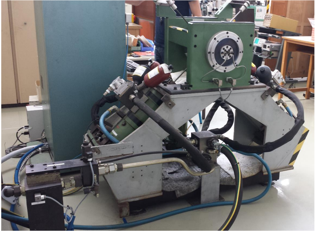
Figure 7-14. “LISE” machine used in the torsional fatigue campaign
