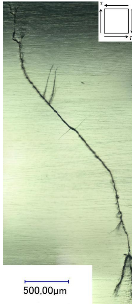
Figure 7-18. Surface crack patterns in the failed specimen: \tau_a = 340 \text{ MPa} ; \tau_m = 500 \text{ MPa} ; N_{\text{cycles}} = 944,988 [Pallarés, 2018B]
