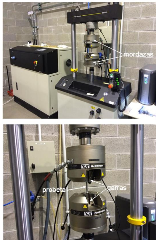
Figure 7-7. Instron 8805 MTB axial fatigue machine located at the E.T.S. de Ingenieros de Bilbao [Avilés, 2018]
