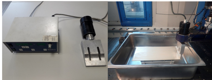
Figure 4. Cleaning equipment (left) and assembly on 3-axis machine (right).
