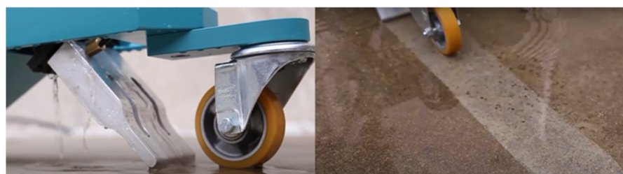
Figure 2. This illustrates non-immersion floor cleaning using the cleaning device. The picture on the left shows the sonotrode tips assembled on a trolley. The picture on the right shows the same device cleaning a dirty floor by sweeping the sonotrode. The difference between the dirty and clean areas is clearly visible to the naked eye.
