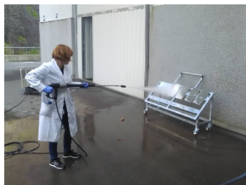
Figure 7. High pressure water jet cleaning at 1.5 m distance.
