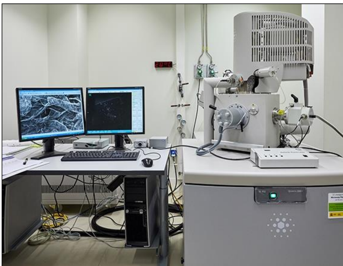
Figure 2.3: FEI Quanta 200 FEG SEM (Themofischer).
