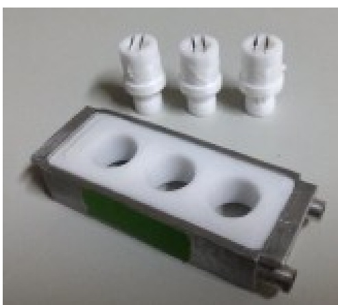
Figure 2.5. Homemade chamber and PTFE circular wells for the formation of GUV attached to a platinum wire.
