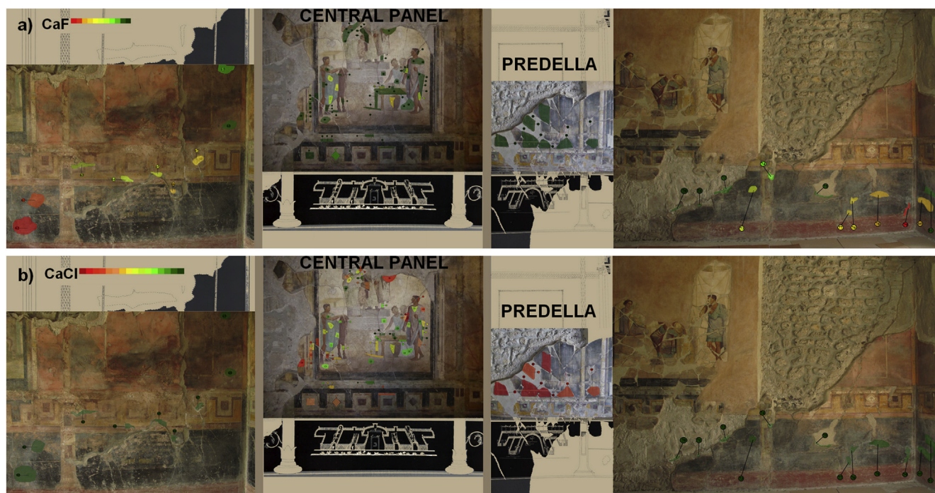
Fig. 2. Qualitative LIBS distribution image of A) CaF and B) CaCl of Room G of the House of the Golden Cupids. Vertical wide lines mark the separation of the north, eastern and south walls. Red areas correspond to the points with higher relative net intensities, while green areas correspond to lower relative net intensities. (For interpretation of the references to color in this figure legend, the reader is referred to the Web version of this article.)
