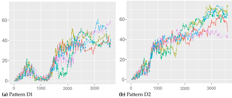
Figure 5.4: Evolution of the total vehicle volume time series in each 60-minute length simulation run for demand patterns D1 (a) and D2 (b). Five simulations for each demand, cover a total duration of 10 simulation hours.
