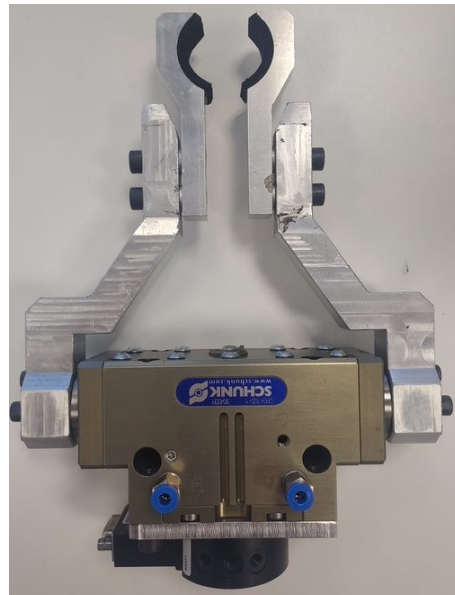
Figure 2. The pneumatic gripper used for grasping the detected objects.
