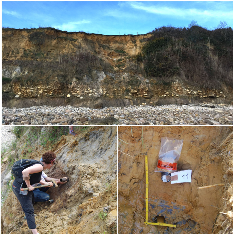
Figure 3. View of the Oyambre outcrop (upper picture) and sampling procedure. Left: metal tubes were introduced into the sediment using a hammer. Right: sample Ploy-11 was obtained by the insertion of a steel tube into the sandy sediment and also collecting extra bags with an adjacent sub-sample. The lower sample (Ploy-10) was collected from a dark, very fine silt layer. [Color figure can be viewed at wileyonlinelibrary.com ]
