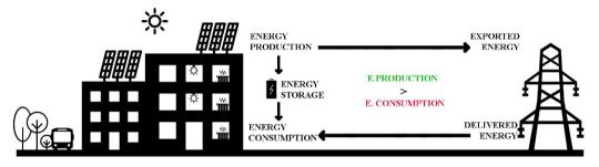
Fig. 1. Graphical explanation of a PED.
