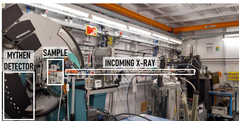
Figure 2.7: MSPD beamline at ALBA synchrotron. The incoming beam tube, the position of the sample and the detector have been highlighted.
