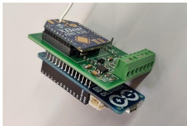
Figure 8. Detail of the Smart Measuring Node prototype board.
