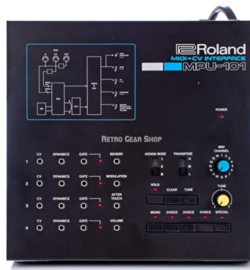
Figura 14. Midi to CV/gate converter Roland MPU-101
