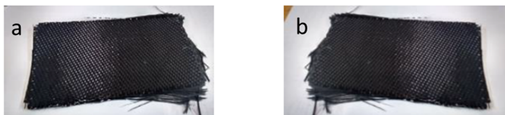
Figure 3. Carbon fiber fabrics after pyrolysis-oxidation process: rCF1 (a) and rCF2 (b).
