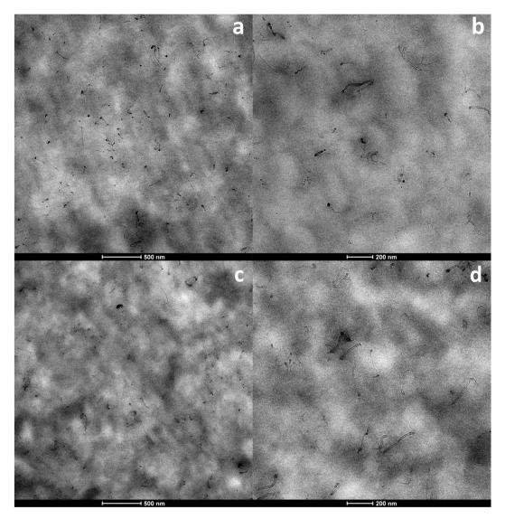
**Figure 5.** TEM micrographs of PA410/Pebax/CNT ternary (**a**,**b**) and PA410/PA6/Pebax/CNT quaternary (**c**,**d**) NCs with a CNT content of 0.4 wt%, at ×14,500 and ×25,000 magnifications.
