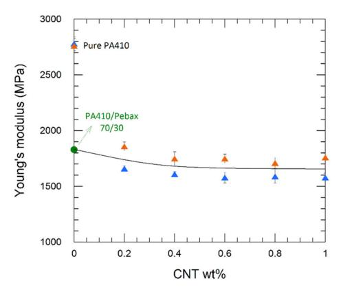
**Figure 9.** Young's modulus of PA410/Pebax/CNT () and PA410/PA6/Pebax/CNT () NCs vs. the CNT content. Pure PA410 and the PA410/Pebax2 70/30 blend have been represented as a reference.
