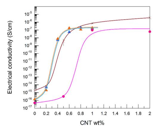
**Figure 8.** Electrical conductivity of PA410/Pebax/CNT () and PA410/PA6/Pebax/CNT () NCs vs. the CNT content. PA410/CNT (**x**) and PA410/PA6/CNT (**•**) systems have been represented as a reference [1].
