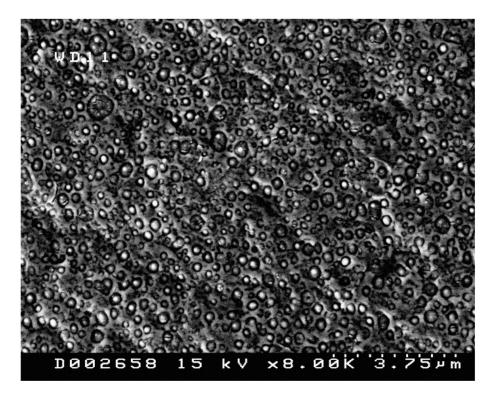
Figure 3. SEM micrograph of unfilled PA410/Pebax 70/30 blend.
