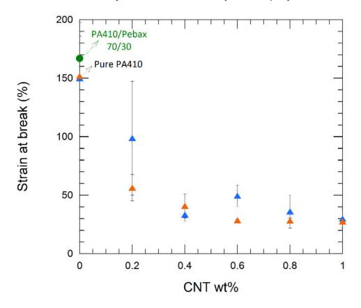
**Figure 11.** Strain at break of PA410/Pebax/CNT (▲) and PA410/PA6/Pebax/CNT (▲) NCs vs. the CNT content. Pure PA410 and the PA410/Pebax2 70/30 blend have been represented as a reference.
