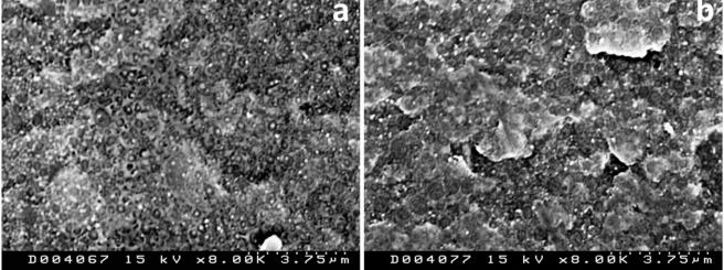
Figure 6. SEM micrographs of PA410/Pebax/CNT NCs: (a) 0.6% CNT; (b) 1% CNT.
