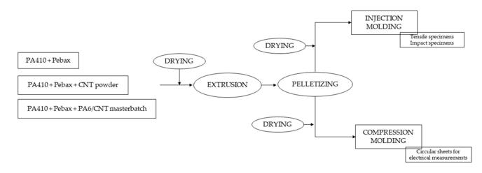
Scheme 1. Schematic representation of the preparation of the materials.
