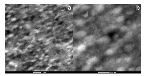
**Figure 4.** TEM micrographs of the PA410/Pebax 70/30 blend: (**a**) At ×5000 magnification; (**b**) at ×14,500 magnification.
