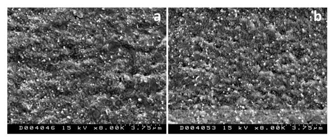
Figure 7. SEM micrographs of PA410/PA6/Pebax/CNT NCs: (a) 0.6% CNT; (b) 1% CNT.
