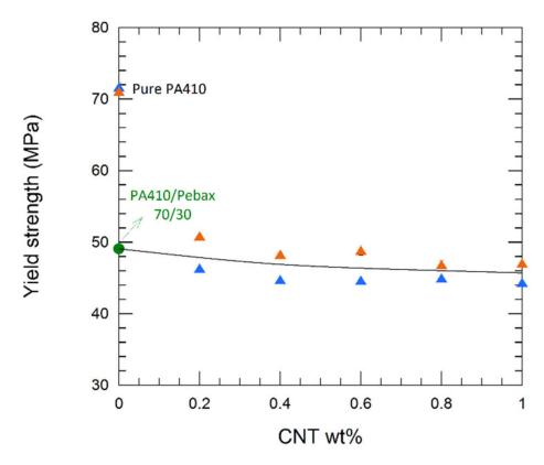
**Figure 10.** Yield strength of PA410/Pebax/CNT () and PA410/PA6/Pebax/CNT () NCs vs. the CNT content. Pure PA410 and the PA410/Pebax2 70/30 blend have been represented as a reference.
