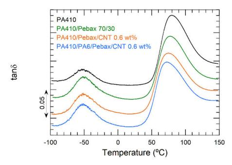
**Figure 1.** DMTA curves of pure PA410, PA410/Pebax 70/30 unfilled blend and, as an example, PA410/Pebax/CNT and PA410/PA6/Pebax/CNT NCs with a 0.6 wt% CNT content. Curves have been shifted in the vertical axis.
