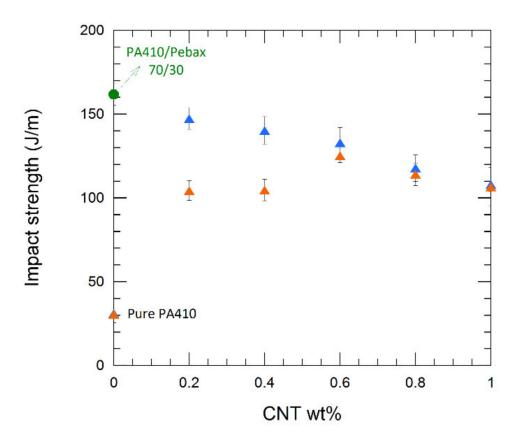
**Figure 12.** Impact strength of PA410/Pebax/CNT (▲) and PA410/PA6/Pebax/CNT (▲) NCs vs. the CNT content. Pure PA410 and the PA410/Pebax2 70/30 blend have been represented as a reference.
