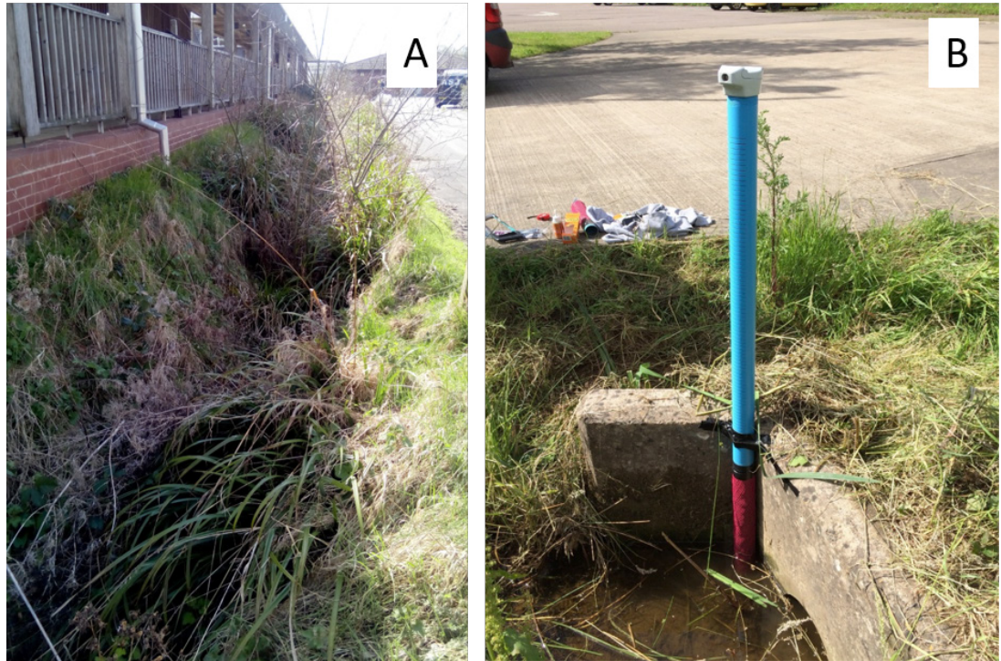
Fig.2. View of the vegetated swale (A) and monitoring equipment (B).
