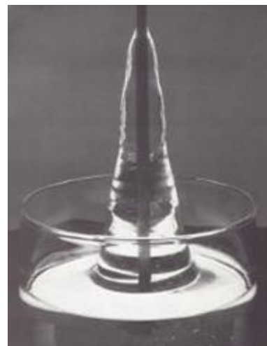
Figure 75. Weissenberg effect example in a high molecular weight PIB and low molecular weight polyisobutylene solution. [120]
