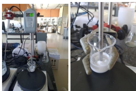
Figure 23. Preparation process of a glycerol-based hydrogel. Close-up of the rotor mixing the hydrogel and its components. Glycerol based mixture.
