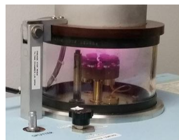
Figure 34. Gold sputtering process. [118]
