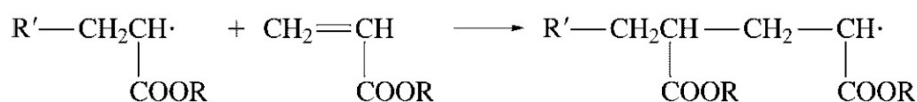
Fig. 1. General FRP propagation mechanism for an acrylate monomer (for BA R = C 4 H 9 ).
