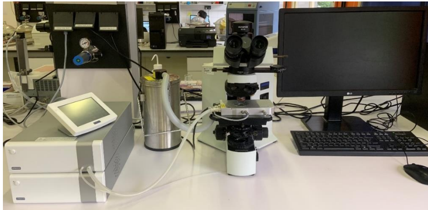
Figure 2.7. Equipment that was used in the lab: the PLOM, the hot stage and the computer.
