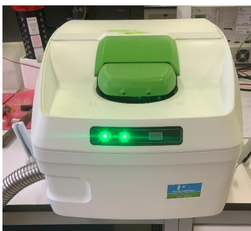
Figure 2.10. DSC Perkin Elmer 8000 calorimeter that was used in the lab.
