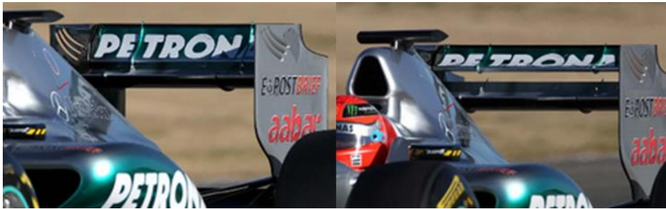
Figure 1-14. DRS closed (left) and open (right) [13]
