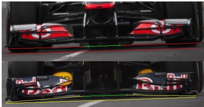
Figure 1-11. Front wing flexing RB7 (bottom) vs MP4-26 (top) [10]
