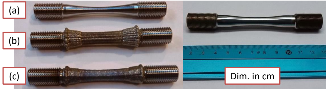
Figure IV.19. Left, coated specimen in different manufacturing stages (a) preform, (b) coated specimen with longitudinal strategy respect to its axis, (c) coated specimen with helix strategy. Right, machined and polished coated specimen. Note the excess material that has been added in each type of strategy to ensure that there is enough material to machining the specimen to the final dimension according to the standard specifications.
