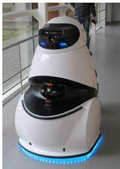
Figure 3. Teknibot is a guide robot that is able to guide its users to a given destination.
