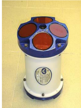
Figure 2.7. An RDI Workhorse ADCP as the ones installed on EuskOOS slope moorings.
