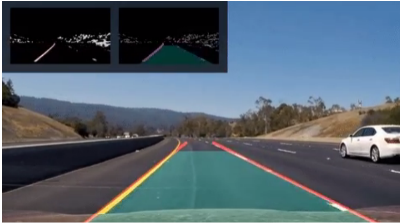
FIGURE 1.2: Video-based ADAS can detect lane marks in almost any visibility condition. Through border detection algorithms and the computation of the perspective, LDW systems can determine if the wheel of the vehicle is stepping over the lane mark by only using a front camera.
