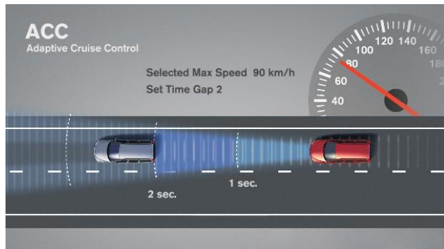
FIGURE 1.1: Representation of an ACC system. Through radar sensing, the red vehicle measures the time gap with the preceding one and adjust its speed to keep it constant.
