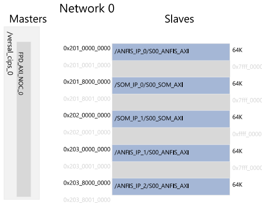
FIGURE 5.4: Structure of the address map of the peripherals integrated in the system. The range of addresses reserved for each peripheral is displayed in blue, while the blank addresses are shown in gray.
