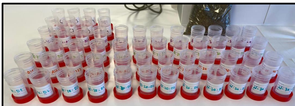
Pots used for assessing DMPSA breakdown in DMP with sterilized and non-sterilized soil
