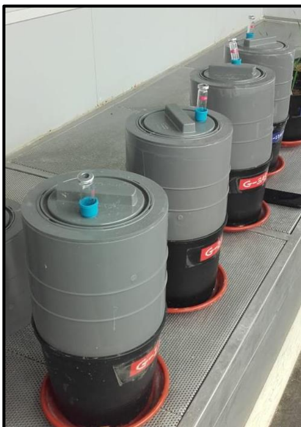
Chambers introduced inside pots for N 2 O emissions sampling
