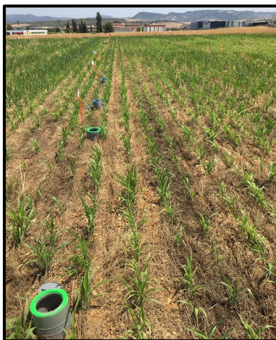
Chambers inserted into the soil for sampling of N 2 O emissions
