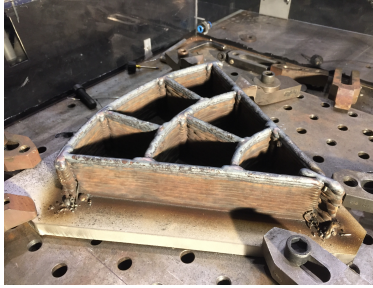
Fig. 6.5: Part manufactured by PAW technology.
