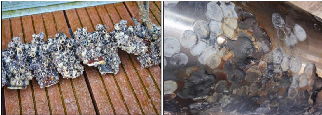
Figure 3-9. Barnacle deposition over a low alloy steel surface at Tecnia's fouling testing facilities in Pasaia (left) and remaining crevice corrosion once bio-organisms are removed (right, courtesy of: boats.com)
