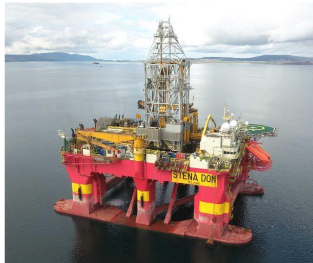
Figure 2-11. ExxonMobil Stena Don semi-submergible unit for offshore Oil&Gas extraction. Source: offshoreenergytoday.com
