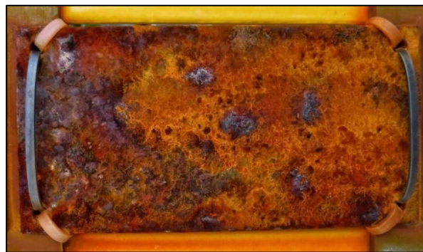
Figure 3-4. Uniform corrosion in a carbon steel sample tested in Tecnia's HARSHLab facility in open seawater.
