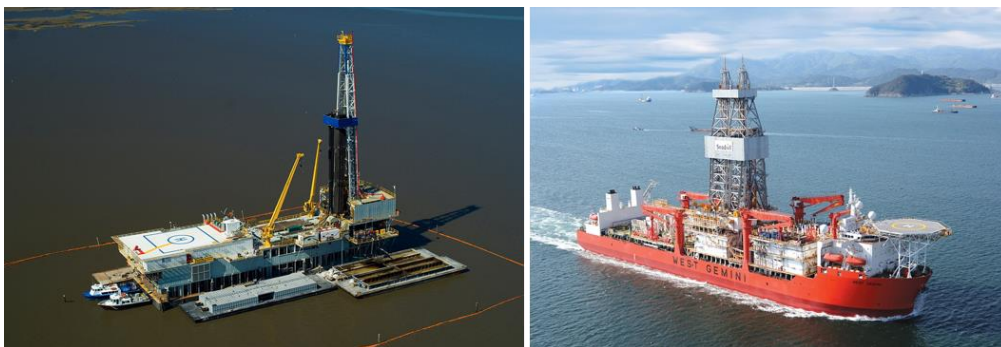
Figure 2-12. Drilling barge for shallow waters (left) and West Gemini Drillingship (right), for offshore locations. Source: media.subsea.org and maritime-connector.com
