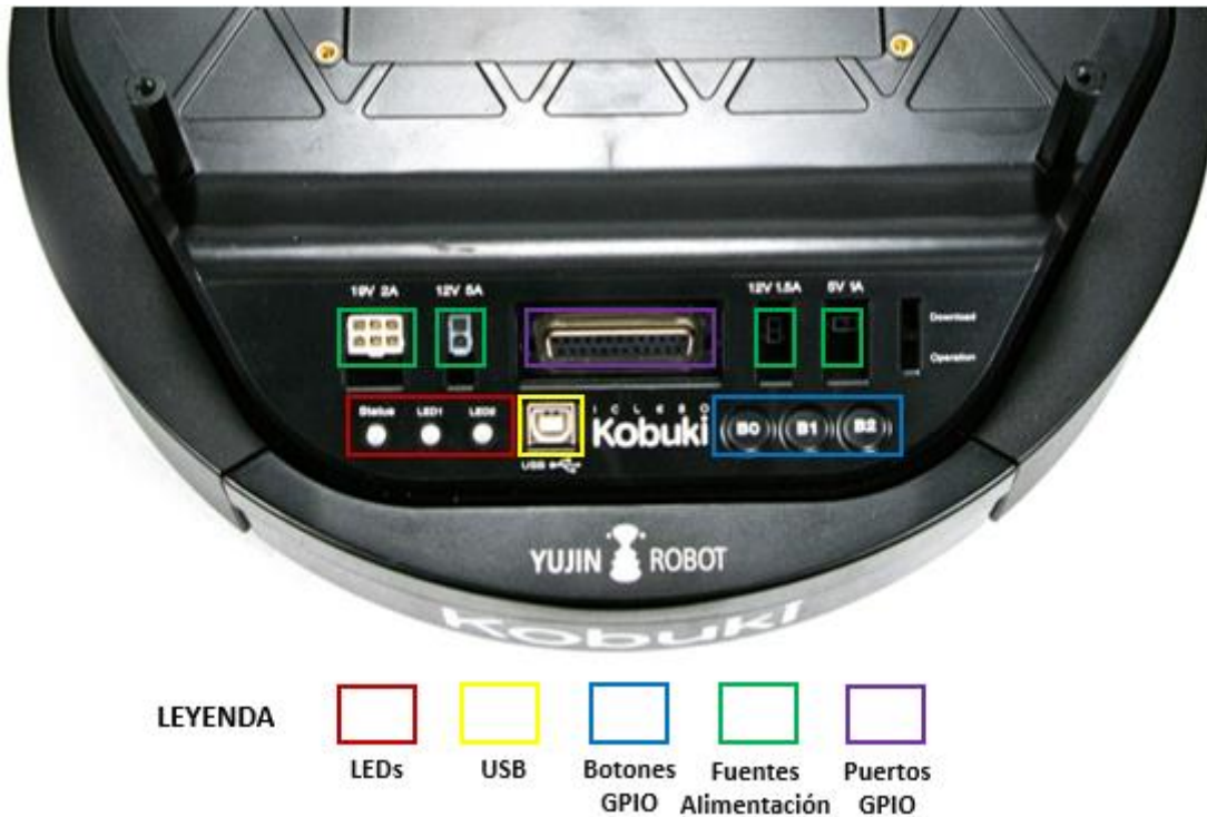
Figura 4.39 Interfaz Hardware del Kobuki iCleBot Turtlebot2
