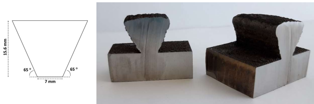
Figure 2. Dove tail structure, cross section.
