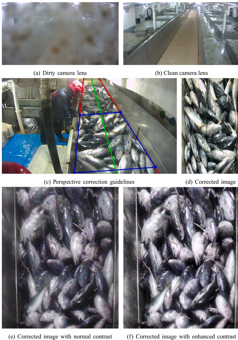
Fig. 2. From left to right and top to bottom: A) Image taken from a camera when it is dirty. This is an extreme example of dirtiness. B) With the camera cleaned. The region of interest is the central conveyor belt. C) Guidelines for perspective correction. The inner area of the blue trapezoid will form the corrected image. D) Same image as before but with the perspective corrected. E) Corrected image with normal contrast and F) corrected image with enhanced contrast. (For interpretation of the references to colour in this figure legend, the reader is referred to the web version of this article.)
