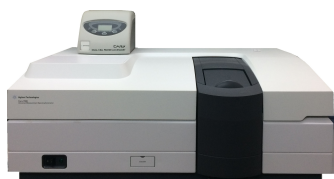
Figure 6.1: Double beam UV-Vis spectrophotometer (Cary 7000).
