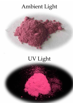
Figure 7.20: Photograph of the bulk LDS 722/AEL powder under ambient and UV light.
