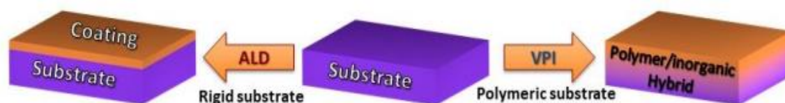
Figure 3. Schematic of the comparison between samples processed by ALD (left) and VPI (right).
