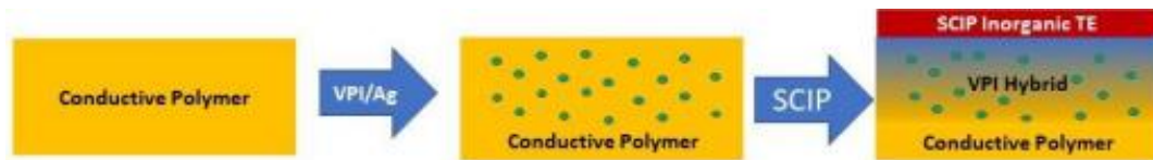
Figure 4. Schematic of material's hierarchy after VPI (blue) and SCIP (red) with created hybrid layer and inorganic coating on top of the polymer substrate.
